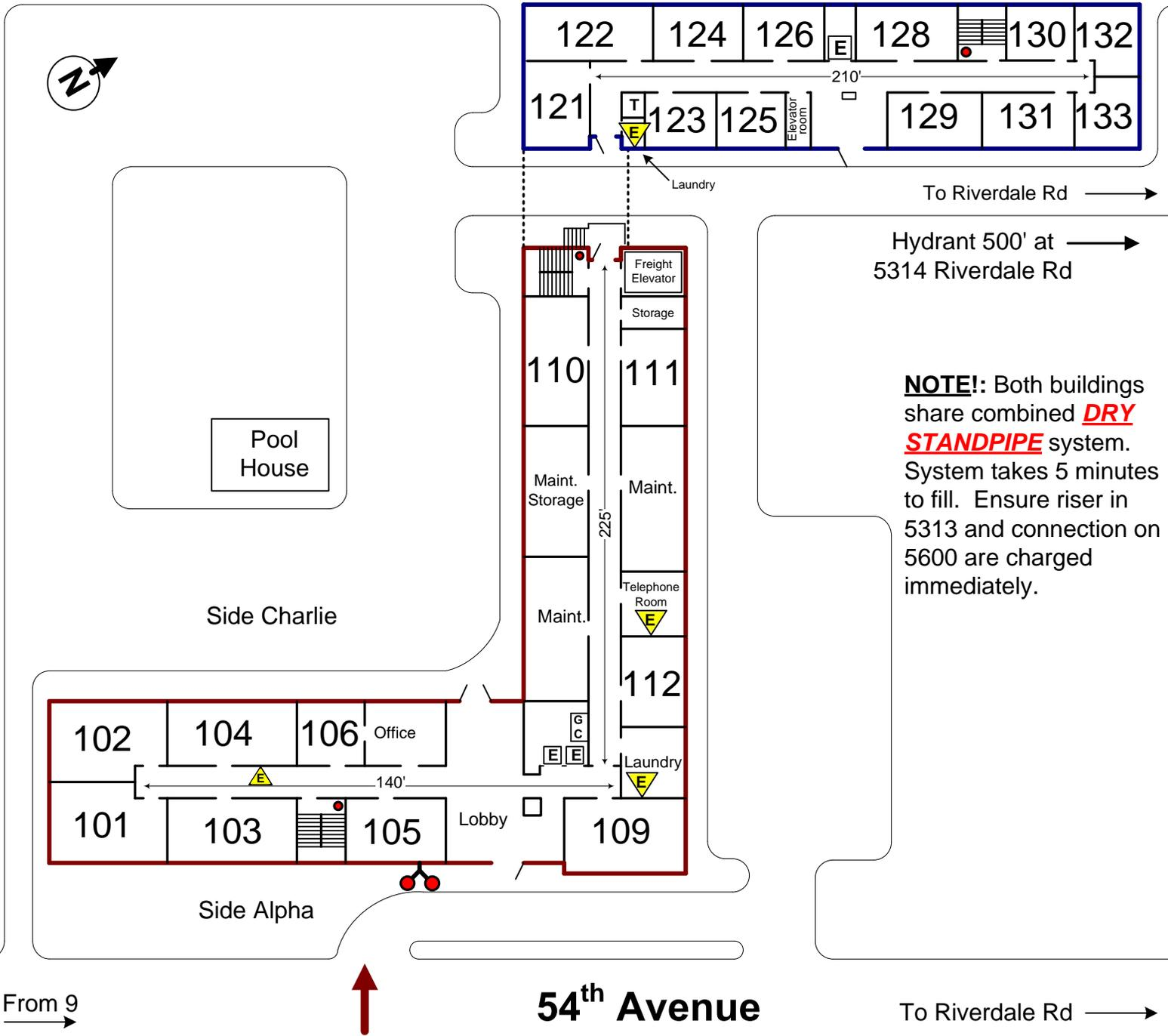
**NOTE!:** Both buildings share combined **DRY STANDPIPE** system. System takes 5 minutes to fill. Ensure riser in 5313 and connection on 5600 are charged immediately.
